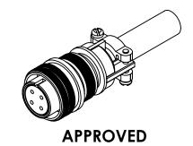
MS High Current Series, Multipin Feedthrough, 4 Pins, 700 Volts, 28 Amps per Pin, 0.094" Moly Conductors, 2.16" Quick Flange
