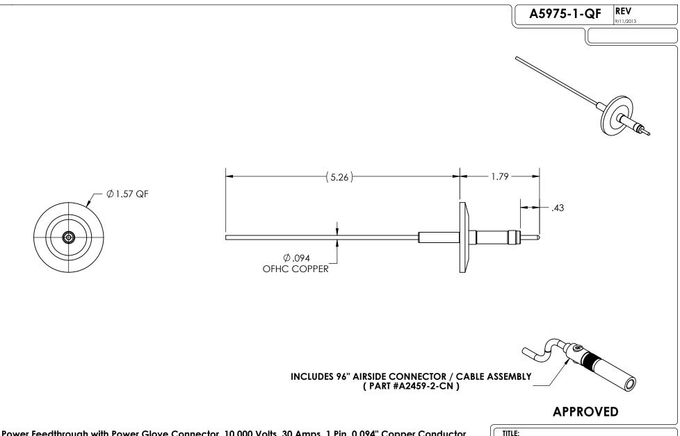
Power Feedthrough with Power Glove Connector, 10,000 Volts, 30 Amps, 1 Pin, 0.094" Copper Conductor 1.57" Quick Flange
