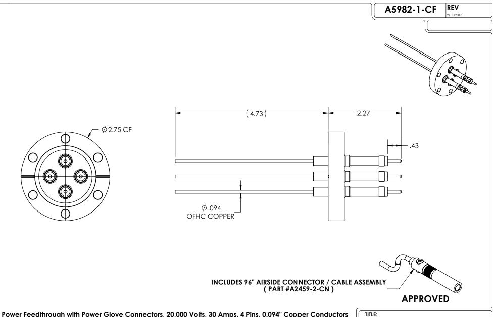
Power Feedthrough with Power Glove Connectors, 20,000 Volts, 30 Amps, 4 Pins, 0.094" Copper Conductors 2.75" Conflat Flange
