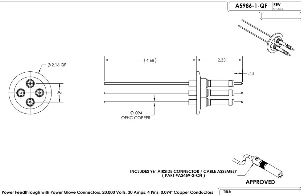
Power Feedthrough with Power Glove Connectors, 20,000 Volts, 30 Amps, 4 Pins, 0.094" Copper Conductors 2.16" Quick Flange
