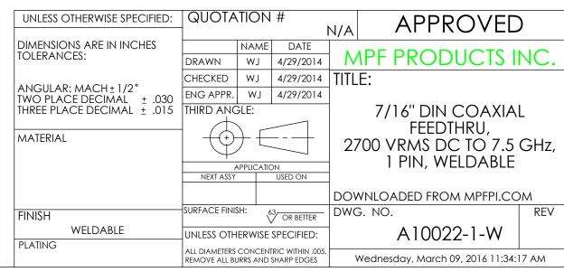
7/16" DIN Coaxial Feedthrough, 50ohm, DC to 7.5 GHz, 2700 VRMS, 100 Watts 0.275" Copper Conductor, 1.375" Weld Adapter.
