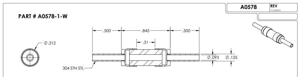
Cryogenic Break, 5KV Isolation, 0.125" Dia Stainless Steel Tube Adapters
